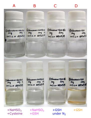
**Fig. 7.** Precipitate formation during the storage of 8.61 mM edaravone in water at  $60^{\circ}$ C for 4 weeks under aerobic condition in the presence of 9.61 mM NaHSO<sub>3</sub> and 4.13 mM cysteine (A); 9.61 mM NaHSO<sub>3</sub> and 4.13 mM GSH (B); 4.13 mM GSH under N<sub>2</sub> atmosphere (C); 4.13 mM GSH (D).
